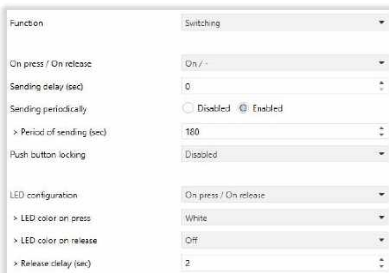
Fig 10 : Switching Function Configuration
