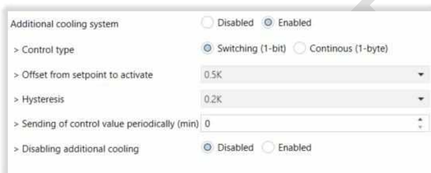
Fig 31 : Additional Cooling System Configuration
