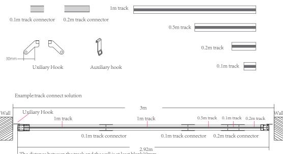
The distance between the track and the wall is at least blank10mm
